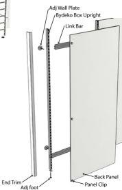
Bydeko Perimeter System uses Bydeko Box Uprights with link bars and/ or panel-clips to carry a variety of different backpanels. Panels can be slotted, printed, wood veneer or melamines, made to order.
